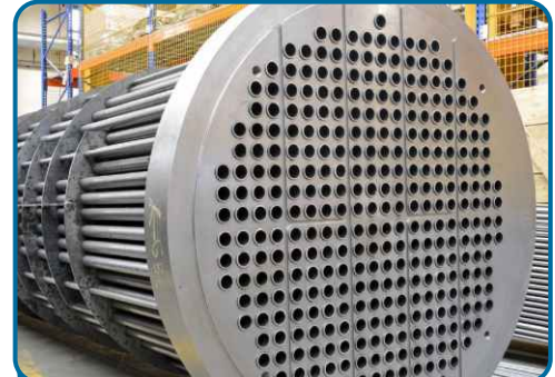
Tube Sheet Thickness : 35-50 mm
